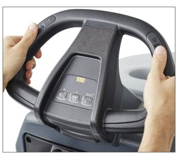
8. Start cleaning by placing the hands on the touch sensors on the handlebar.
