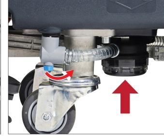
15. Clean the filter:A) Close the solution valve under the machine.B) Remove the transparent cover and the gasket, then remove and clean the filter inside.C) Reassemble the filter.
