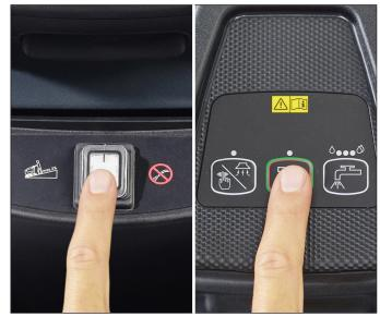
6. Turn the main switch to "I", press the main button (LED on) to start the machine.
