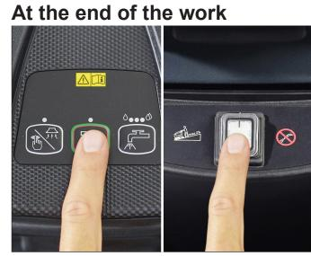
10. Press the main button (LED off) to stop the machine, turn the main switch to "0". Disconnect the power supply plug from the electrical mains
