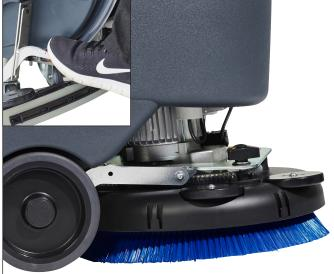
12. Lift the brush deck by pressing the pedal, remove and clean the brush/ pad.
