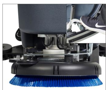
Place the brush or the pad-holder under the deck. Use the appropriate brush to clean the floor. Lower the deck by pressing the pedal deck.
