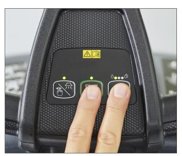
7. For sensitive floors the brush/pad can be pre wetted with solution before starting to work to avoid marks. Press the main button and the solution button simultaneously for 10/20 seconds before starting to work.
