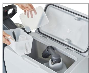
14. Empty the debris tray and clean/wash the recovery tank inside.
