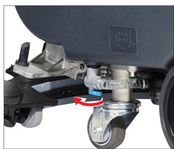
2. Make sure the solution valve under the machine is open.
