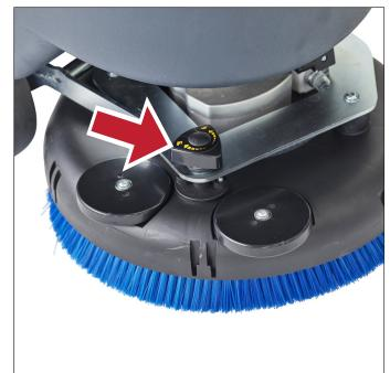
1. To adjust machine direction turn front knob until machine is working straight.
