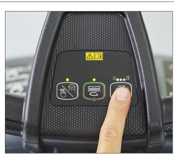
Press the solution button to adjust the solution flow to the cleaning needs.
