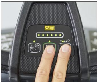
9. For sensitive floors the brush/pad can be pre wetted with solution before starting to work to avoid marks. Press the main button and the solution button simultaneously for 10/20 seconds before starting to work.
