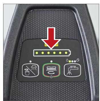
2. Check if there isn't any brush motor overload indicated by Led's blinking.
