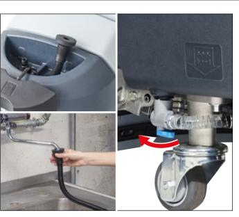
2. Fill the tank with clean water and dosage a suitable detergent according to the specifications. The water temperature must not exceed 40 °C. Make sure the solution valve under the machine is open.
