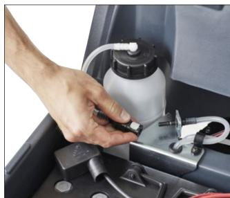
3. (if machine have detergent mixing) Fill the bottle with a detergent suitable for cleaning machines (highly concentrated and low foaming).
