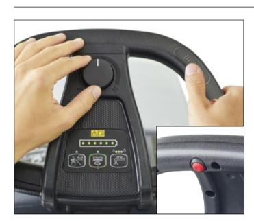
11. (for drive model) If necessary, adjust the maximum speed with the speed adjustment knob. For reverse, press the rear button of the handle together with one hand on any of the touch sensors.
