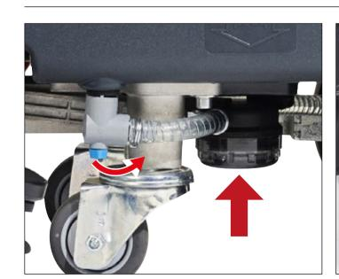
16. Clean the filter:A) Close the solution valve under the machine.B) Remove the transparent cover and the gasket, then remove and clean the filter inside.
