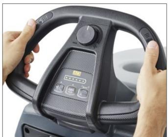
10. Start cleaning by placing the hands on the touch sensors on the handlebar.
