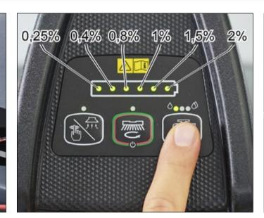
4. (if machine have detergent mixing) Activate machine with battery led only. Change the percentage of detergent in the cleaning solution by pressing the solution button for 2 sec., than toggle the battery led to desired setting by pushing the solution button.
