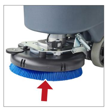
2. Check if the brush are correctly installed and not worn out or if there are external materials avoiding brush rotating.
