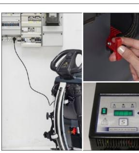
19. Charge the batteries: Connect the battery charger cable to the electrical socket.
