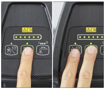
8. Press the main button again (with LED on) to start the machine, press the vacuum button and the main button simultaneously for 1 sec. to engage the brush to the deck hub.
