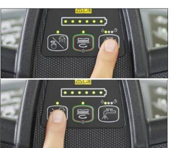
12. Press the solution button to adjust the solution flow to the cleaning needs.
