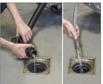
14. Empty the recovery tank with the hose. Then empty the solution tank with the transparent hose.
