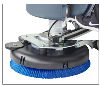
6. Place the brush or the pad-holder under the deck. Use the appropriate brush to clean the floor. Lower the deck by pressing the pedal deck.
