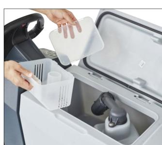
15. Empty the debris tray and clean/wash the recovery tank inside.
