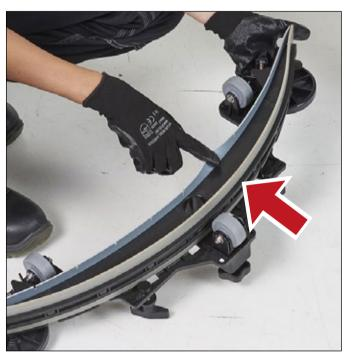
3. Check if squeegee blades are damaged 4. Check the lid gasket is in good and or dirty.
