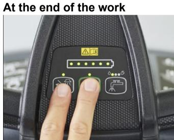
13. Stop working. Lift squeegee and press the main switch to turn machine off but with battery led still on. Lift the brush deck by pressing the pedal. To disengage the brush, press the vacuum button and the main button simultaneously for 1 sec..
